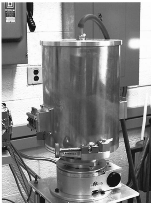
FIG. 2. The detector chamber mounted on a conventional x-ray tube at the Michigan State University. The chamber is hinged on a Huber goniometer for adjustment.
