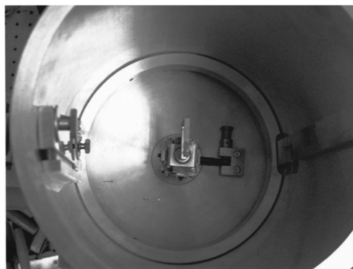
FIG. 3. View of the inside of the chamber with sample holder and support for imaging plate.
