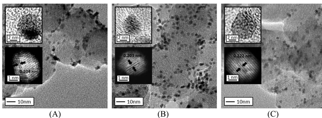
**Figure 2.** TEM images of (A)  $\text{Pt}_{31}\text{Ru}_{69}/\text{C}$ , (B)  $\text{Pt}_{49}\text{Ru}_{51}/\text{C}$ , and (C)  $\text{Pt}_{75}\text{Ru}_{25}/\text{C}$  after thermal treatment. Insets: (top) HR-TEM images and (bottom) HAADF-STEM images of the respective catalysts.
