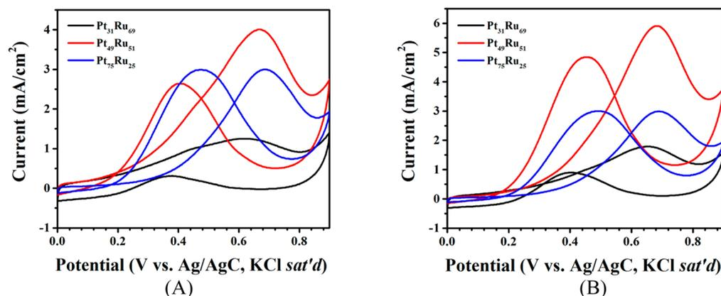
**Figure 6.** CV curves for (A) fresh Pt<sub>n</sub>Ru<sub>100-n</sub>/C ( $n = 31, 49,$  and  $75$ ) catalysts and (B) the same catalysts after 30 potential cycles. Electrode, glassy carbon ( $0.07 \text{ cm}^2$ ) inked with  $5 \mu\text{g}$  of catalyst; electrolyte,  $0.1 \text{ M HClO}_4$  with  $0.5 \text{ M ethanol}$  saturated with  $\text{N}_2$ ; scan rate,  $50 \text{ mV/s}$ .
