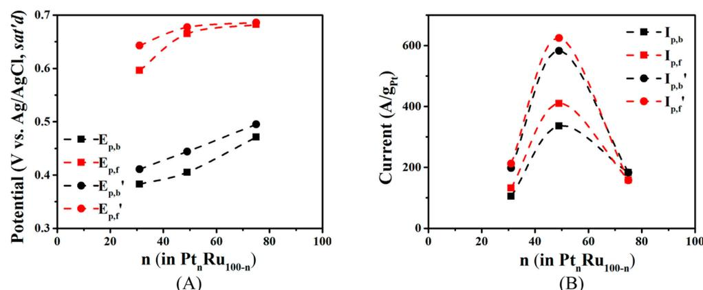
**Figure 7.** (A) EOR peak potentials for the fresh catalysts ( $E_{p,b}$  and  $E_{p,f}$ ) and the same catalysts after 30 potential cycles ( $E_{p,b}'$  and  $E_{p,f}'$ ). (B) EOR peak currents for the fresh catalysts ( $I_{p,b}$  and  $I_{p,f}$ ) and the same catalysts after 30 potential cycles ( $I_{p,b}'$  and  $I_{p,f}'$ ). Electrolyte,  $0.1 \text{ M HClO}_4$  with  $0.5 \text{ M ethanol}$  saturated with  $\text{N}_2$ ; scan rate,  $50 \text{ mV/s}$ . Data extracted from Figure 6.
