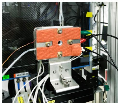
**Figure 8.** Setup of an ethanol vapor fuel cell for in situ HE-XRD/PDF/EDX measurements. Ethanol vapor was carried by  $\text{N}_2$  at 50 mL/min and introduced into the anode half cell, and 3%  $\text{H}_2$  balanced by  $\text{N}_2$  with a flow rate of 50 mL/min was introduced into the cathode half cell, establishing a DHE for the half-cell measurements.
