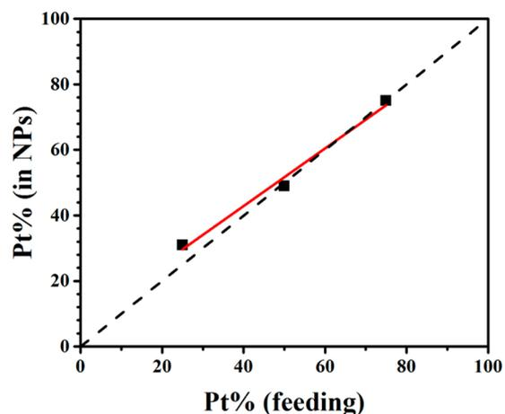
**Figure 1.** Plot of Pt composition in PtRu NPs (from ICP-AES analysis) vs synthetic feeding composition. The dashed line represents a 1:1 relationship. The solid line represents the linear fitting to the actual nanoparticle data (slope = 0.88,  $R^2 = 0.978$ ).
