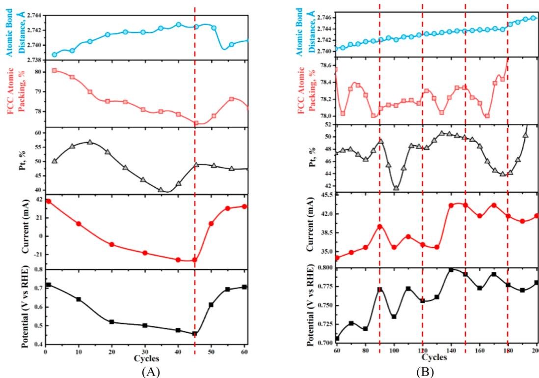
**Figure 11.** Relationship between EOR  $E_{p,b}$  and  $I_{p,b}$  and the in situ evolution of the Pt percentage, fcc atomic packing percentage, and atomic bond distance for  $Pt_{49}Ru_{51}/C$  in the MEA of an ethanol vapor fuel cell (see Figure 8): (A) first 60 cycles and (B) cycles 60–200. Data were extracted from Figures 9 and 10.
