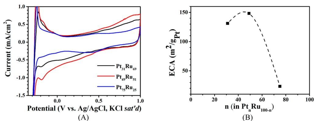
**Figure 5.** (A) CV curves and (B) ECA plot for Pt<sub>n</sub>Ru<sub>100-n</sub>/C ( $n = 31, 49,$  and  $75$ ) catalysts. Electrode, glassy carbon ( $0.07 \text{ cm}^2$ ) inked with  $5 \mu\text{g}$  of catalyst; electrolyte,  $0.1 \text{ M HClO}_4$  saturated with  $\text{N}_2$ ; scan rate,  $50 \text{ mV/s}$ .
