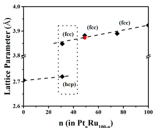
**Figure 3.** Lattice parameters (calculated from PDFs) vs composition for  $\text{Pt}_n\text{Ru}_{100-n}$  ( $n = 31, 49,$  and  $75$ ). Dashed lines are the fitting relationships between metal and PtRu NPs. The dashed box for  $\text{Pt}_{31}\text{Ru}_{69}$  indicates the co-existence of hcp and fcc phases. Black squares are data extracted from a recent report.<sup>25</sup> The red circle indicates data extracted from the study reported herein.
