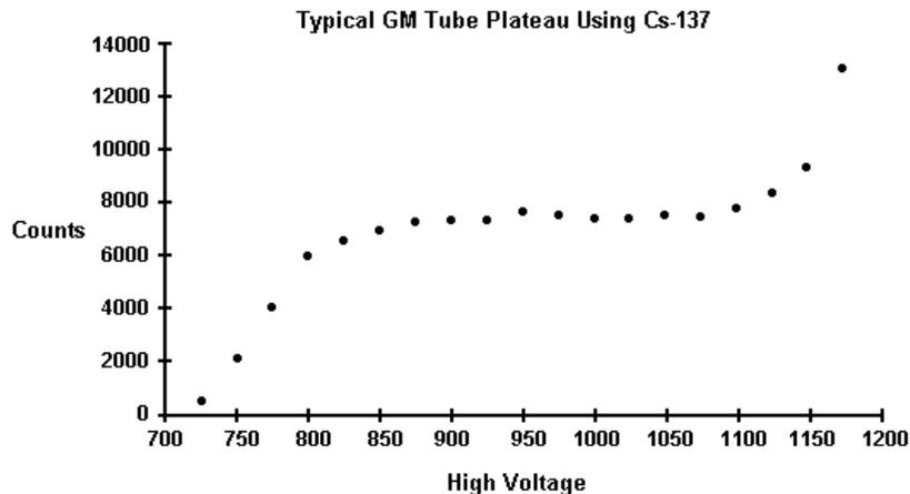
**Figure 2.** A typical GM tube plateau. Notice that the counts form a relatively *flat* region on the graph between 850 and 1150 volts. The center of this area is at approximately 950 volts and is the recommended operating voltage for this detector. However, any voltage in this *flat* region would be acceptable. Also, notice that the counts increase rapidly as the high voltage nears its upper limit. This indicates that the tube is entering its breakdown region.
