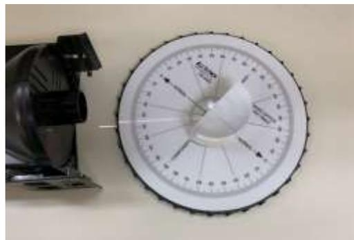
3. Set the D-shaped plate in the marked outline on the spinning table, with its frosted side of against the table.
