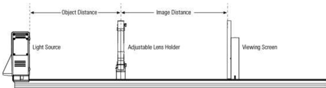
7. Slide the lens holder 5 cm farther down the track, away from the light source. (Do not change the light source position.)
