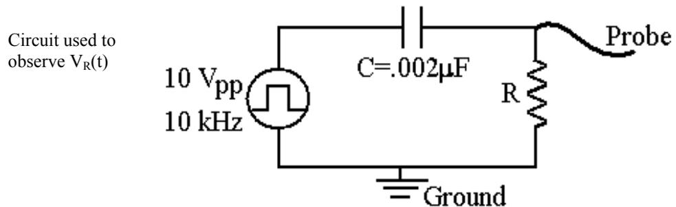
Observe the voltage across the resistor with the oscilloscope and sketch the signal for the three R values.
