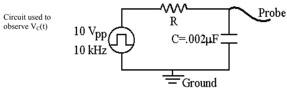
3. Interchange R and C (as shown in the circuit below) so that the voltage across R can be observed and proper ground connections can still be made.
