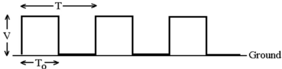
The period of the square wave is  $T = 2T_0$ . Note that it has a positive D.C. offset of  $V/2$  so that it does not go below ground.
