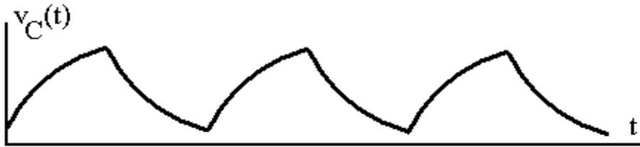
The current during charging and discharging can be found by examining the rate at which charge changes with time.
