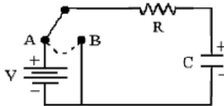
While the switch is at A the capacitor charges up according to the equation (Kirchhoff's voltage law):
