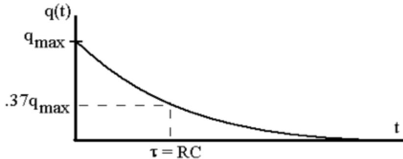
The time required for the charge to drop to 37% of its maximum value is again taken to be the time constant  $RC$ .
