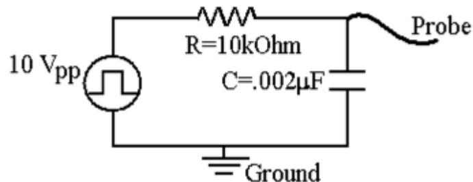
Observe the voltage across the capacitor with the oscilloscope. In order to make an accurate measurement it will be necessary to first vary the frequency of the square wave so that the capacitor becomes just completely charged in time  $T_0$ . Then adjust the time scale on the oscilloscope (sec/div) so that this charging pulse is displayed over a major portion of the screen. Record this oscilloscope setting.
