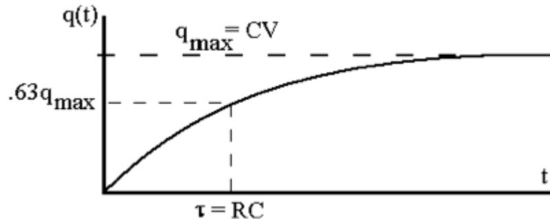
The charge on the capacitor starts out at zero and approaches a maximum value  $CV$ . The time constant  $\tau = RC$  is the time required for the capacitor to change to  $\approx 63\%$  of its maximum value.
