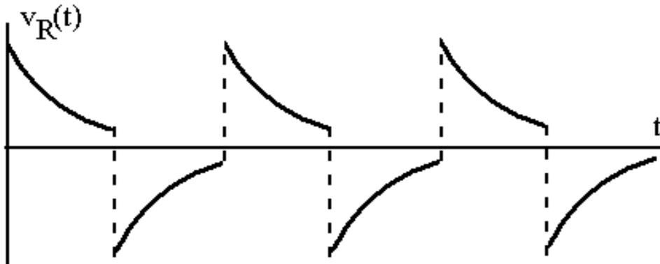
If  $T_0$  is not long enough (compared with the  $RC$  time constant) to allow complete charging and discharging of the capacitor, then the curves for  $V_C(t)$  and  $V_R(t)$  will have shapes that do not show exponential behavior as clearly as those drawn above.
