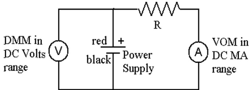
3. Connect a battery, digital multimeter, and resistor in series to form the circuit shown below. This time the digital multimeter measures the current through the resistor. Be sure that your circuit is connected properly. The multimeter is protected against large currents only by a fuse. In this version of the circuit the VOM is used to monitor the voltage across the battery.
