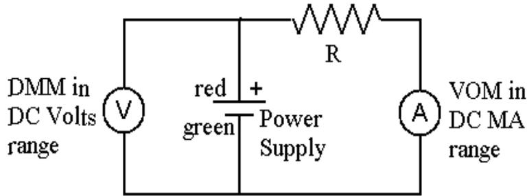
negative currents up to 1.5 mA. To obtain the negative values of current simply reverse the leads attached to the power supply.
