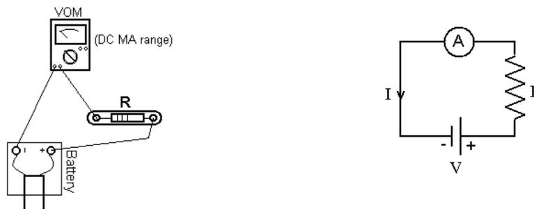
In the diagram the current I is opposite to the direction of the electron current flow. This convention for showing current direction is common in all technical disciplines.
