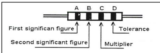
For example, if the bands on a resistor are red (A), black (B), orange (C), and silver (D), then the resistance is  $20 \times 1,000 = 20,000 \Omega$  or  $20 \text{ k}\Omega$ , and the tolerance is  $2,000 \Omega$  (ten percent of  $20,000 \Omega$ ).
