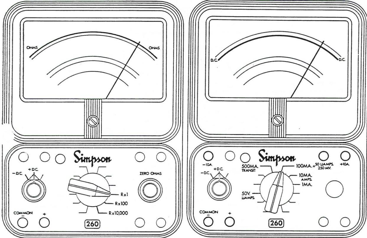
Jacks and switch positions for measuring resistance
