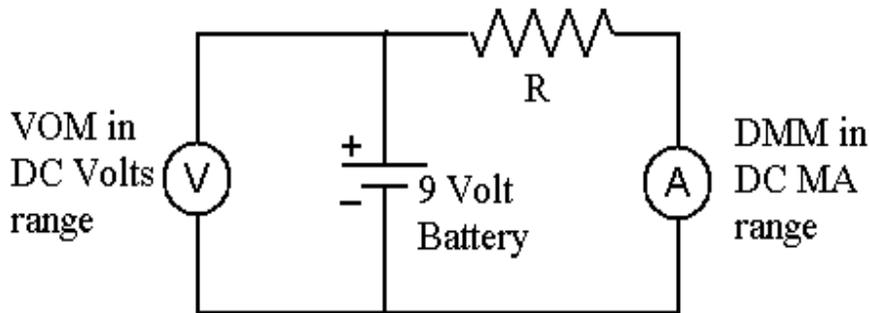
4. Replace the battery by the power supply set to a voltage output equal to the battery voltage when zero current is being drawn from it. Again use the digital multimeter to measure I and use the VOM to measure V.
