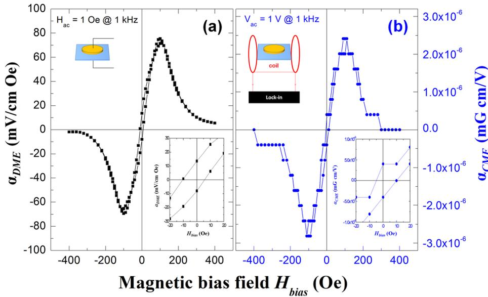
FIG. 4. (a) DME coefficient ( $\alpha_{DME}$ ) and (b) CME coefficient ( $\alpha_{CME}$ ) for BT-0.725BFO/Ni laminates as a function of  $H_{bias}$ . Insets are schematic diagrams of DME and CME samples and expanded views of  $\alpha_{ME}-H_{bias}$  hysteresis to clearly show the remnant  $\alpha_{DME}$  and  $\alpha_{CME}$  at zero  $H_{bias}$ .
