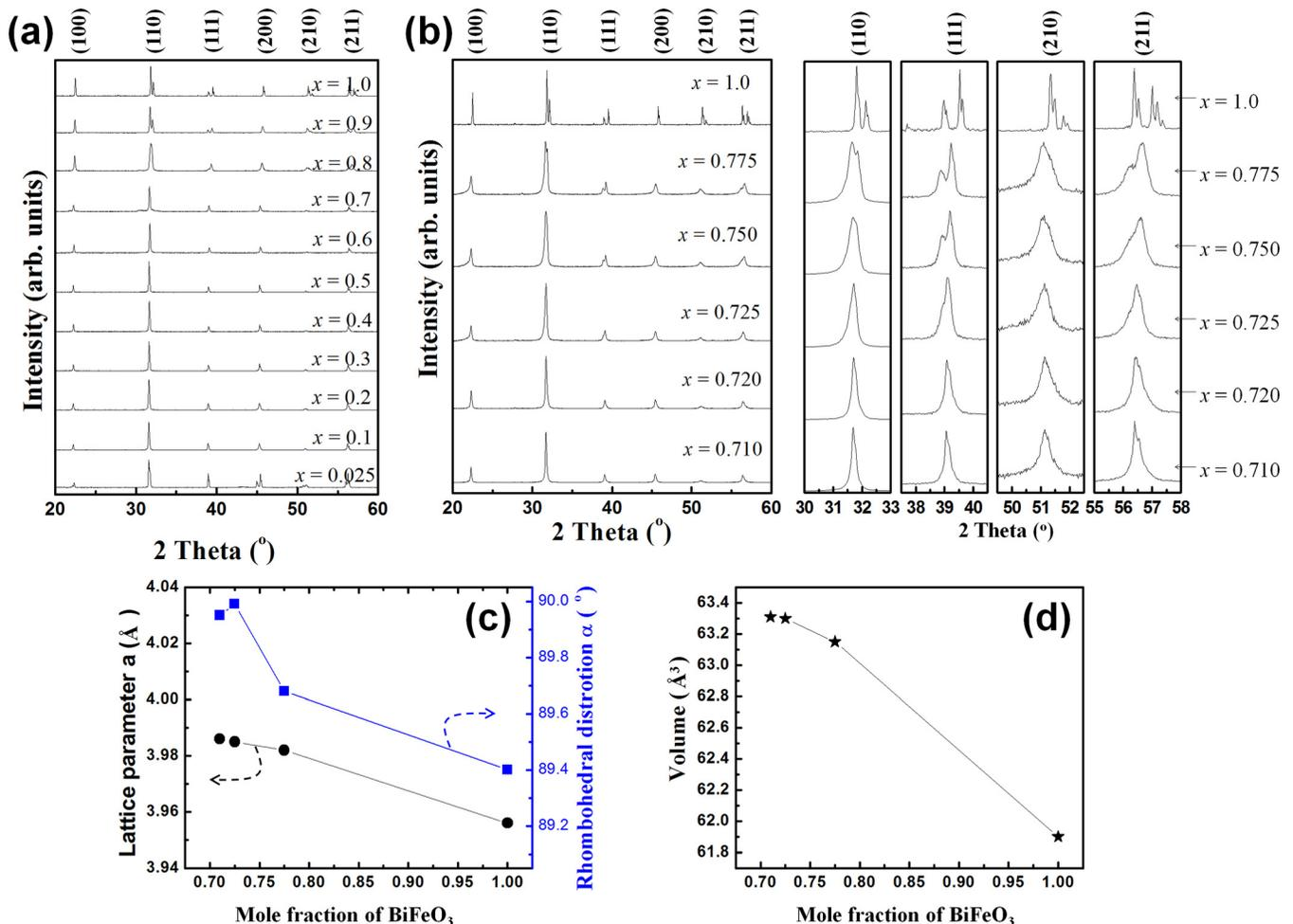
FIG. 1. X-ray diffraction pattern for BT- $x$ BFO ceramics (a) with  $x = 0.025 - 1.0$  and (b) with  $x = 0.710 - 0.775$  and 1.0, (c) lattice parameter and rhombohedral distortion angle and (d) volume of unit cell for BT- $x$ BFO ceramics with  $x = 0.710 - 0.775$  and 1.0.
