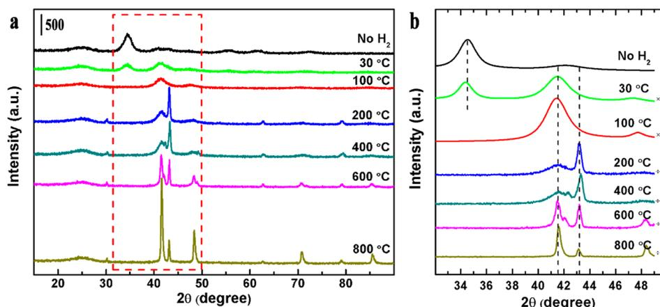
**Figure 2.** (a) XRD patterns for samples of PdCu/C catalysts as a function of  $H_2$  thermal treatment conditions. (b) A magnified view of the boxed region in panel a for a better visual comparison.
