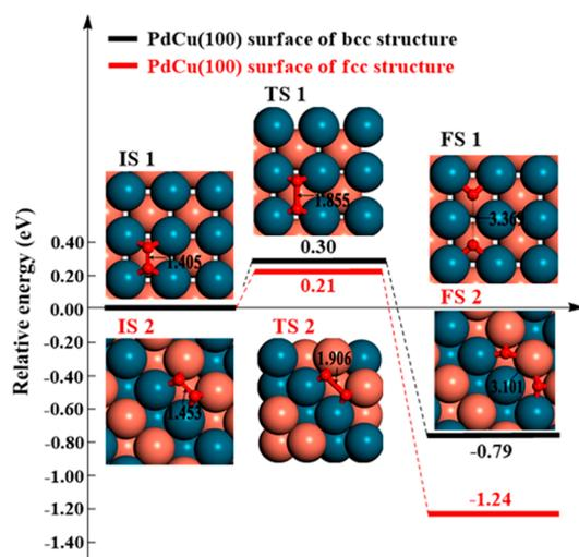
**Figure 6.** Energetics of the O–O bond cleavages of O<sub>2</sub> molecule on the PdCu(100) surface of bcc and fcc crystal structure. The key geometrical parameters are provided in angstroms. The big blue and coral balls are palladium and copper atoms, respectively; small red balls are O atoms.
