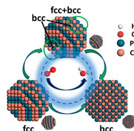
structure prepared by an unusually low thermochemical treatment temperature (100 °C) exhibits higher ORR activity than that with a mixture of fcc and bcc structures.
