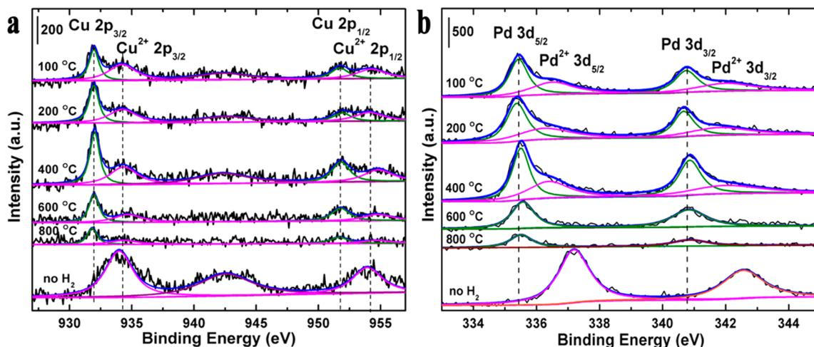
**Figure 4.** XPS spectra and deconvoluted peaks for PdCu/C NPs thermally treated with H<sub>2</sub> at different temperatures in regions of (a) Cu 2p and (b) Pd 3d.
