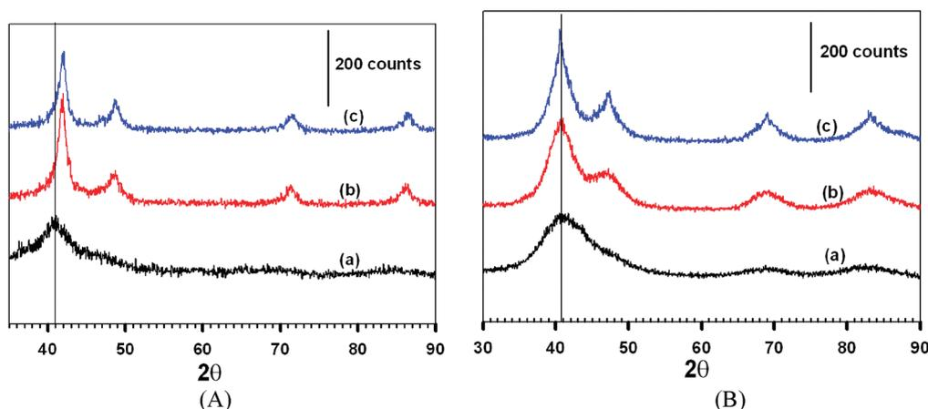
**Figure 5.** XRD patterns: (A)  $\text{Pt}_{25}\text{Ir}_{20}\text{Co}_{55}/\text{C}$  catalysts treated at 400 °C (a), 650 °C (b), and 926 °C (c) (44–50 wt %). (B)  $\text{Pt}_{61}\text{Ir}_{24}\text{Co}_{15}/\text{C}$  catalysts (21–24 wt %) treated at 400 °C (a), 600 °C (b), and 800 °C (c).
