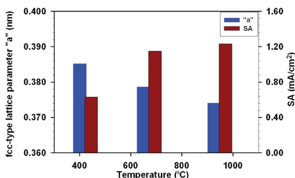
**Figure 9.** Comparison of the ORR specific activity and the fcc-type lattice parameter “a” as a function of thermal treatment temperatures for Pt<sub>25</sub>Ir<sub>20</sub>Co<sub>55</sub>/C catalysts.
