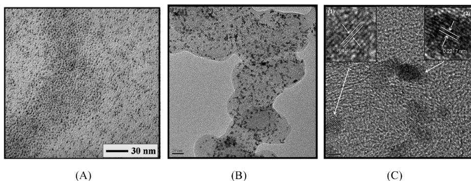
**Figure 2.** (A) TEM for a sample of as-synthesized  $\text{Pt}_{25}\text{Ir}_{20}\text{Co}_{55}$  nanoparticles ( $2.2 \pm 0.2$  nm). (B) TEM (scale bar = 20 nm) and (C) HR-TEM (scale bar = 2 nm) for a sample of  $\text{Pt}_{25}\text{Ir}_{20}\text{Co}_{55}/\text{C}$  catalyst treated at 400 °C. Inset: lattice fringes of (111) for the supported nanoparticles.
