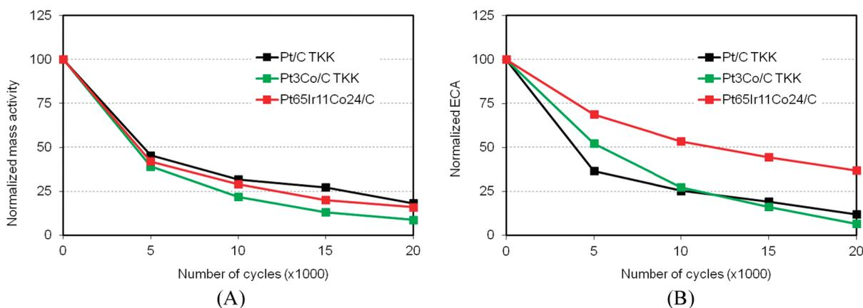
**Figure 10.** Plots of normalized mass activities (A) and ECA values (B) as a function of the number of potential cycles (ranging from 0 to 20,000 cycles) for different catalysts upon potential cycling.
