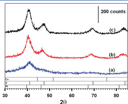
**Figure 3.** XRD patterns of the catalysts: (a)  $\text{Pt}_{25}\text{Ir}_{20}\text{Co}_{55}/\text{C}$ , (b)  $\text{Pt}_{40}\text{Ir}_{28}\text{Co}_{32}/\text{C}$ , and (c)  $\text{Pt}_{65}\text{Ir}_{11}\text{Co}_{24}/\text{C}$  treated at 400 °C (44–52 wt %). Bottom: Standard  $2\theta$  peaks of Pt, Ir, and Co.
