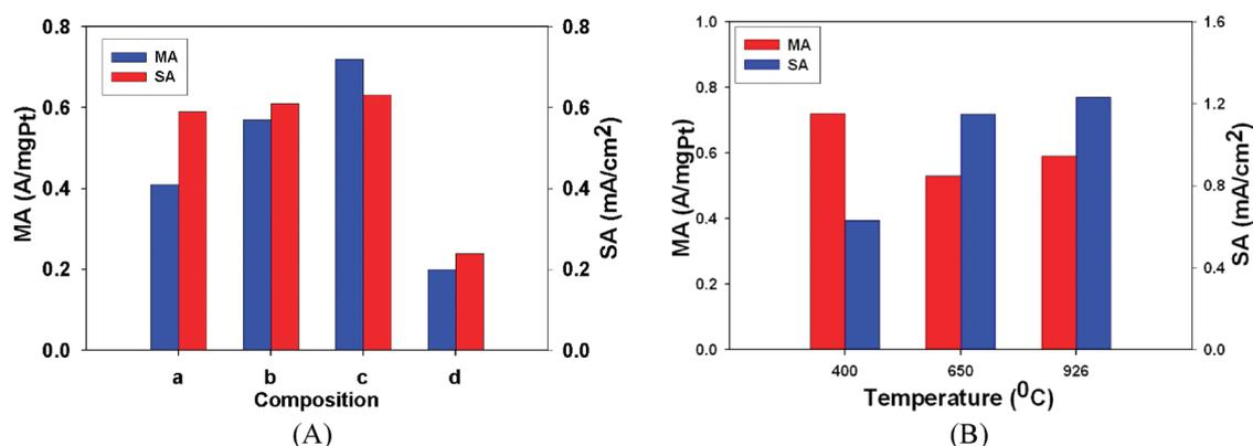
**Figure 8.** Comparison of mass activity (MA) and specific activity (SA) data for catalysts with different compositions. (A) (a) Pt<sub>65</sub>Ir<sub>11</sub>Co<sub>24</sub>/C, (b) Pt<sub>40</sub>Ir<sub>20</sub>Co<sub>32</sub>/C, (c) Pt<sub>25</sub>Ir<sub>20</sub>Co<sub>55</sub>/C, and (d) Pt/C (TKK, 50% wt.); (B) Pt<sub>25</sub>Ir<sub>20</sub>Co<sub>55</sub>/C catalysts treated at different temperatures.
