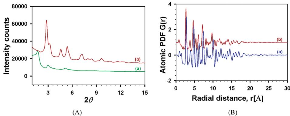
**Figure 4.** HE-XRD patterns for  $\text{Pt}_{25}\text{Ir}_{20}\text{Co}_{55}/\text{C}$  treated at 400 °C: (A) The intensity plots comparing  $\text{Pt}_{25}\text{Ir}_{20}\text{Co}_{55}/\text{C}$  (b) with pure carbon (a); (B) atomic PDFs versus radial distance,  $r$  (in Å), for  $\text{Pt}_{25}\text{Ir}_{20}\text{Co}_{55}/\text{C}$  (b) and pure Pt standard (a).
