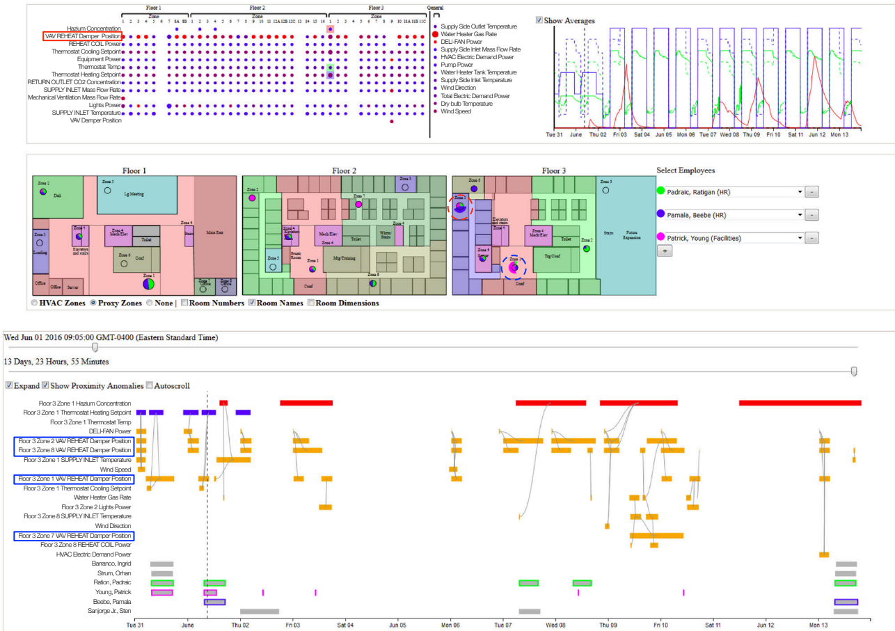
Figure 1: The overview of our visual analytics system. The HVAC view (including dot-matrix plot and line graph), proximity view, and event view are shown at the top, middle, and bottom, respectively. Anomalies related to the hazium concentration spikes at F3Z1-HVAC are linked in the event view.
