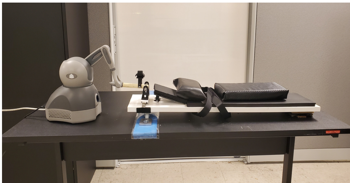
Figure 4. Custom-made portable arm restraint table setup.
