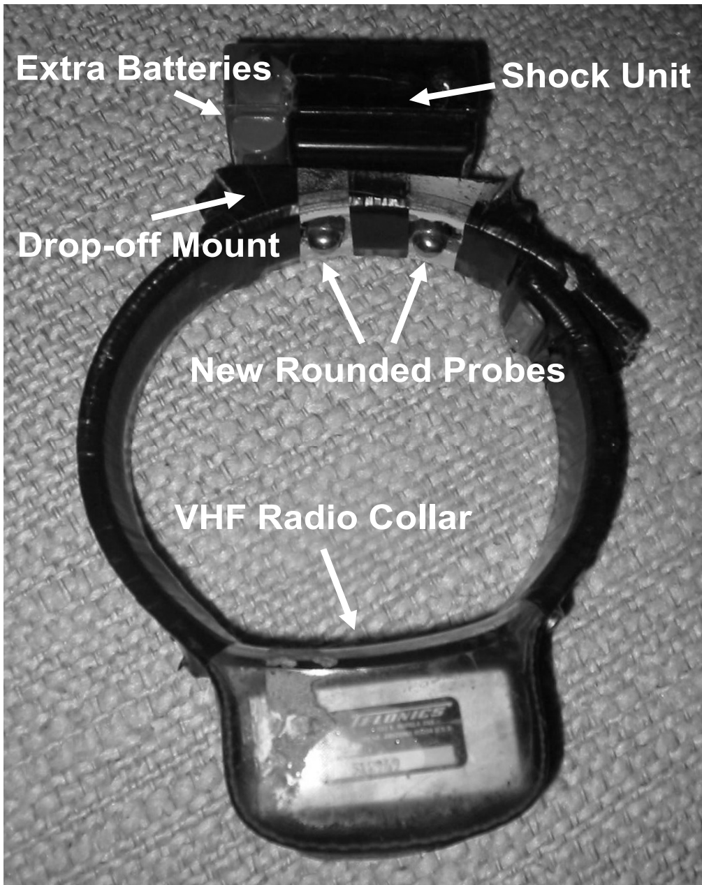
New collar design used in trial #3 with rounded probes, rounded and taped inner collar edges, externally mounted batteries, and drop-off design.
