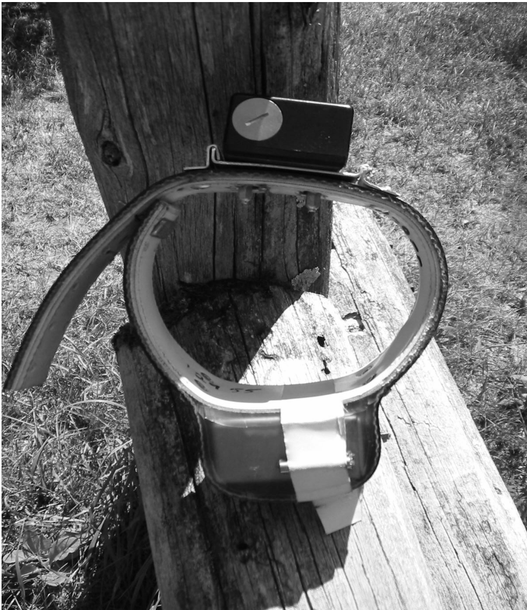
Shock collar design used in trial #3. Includes shock unit with 2 cm probes mounted on the back of a Telonics VHF Radio Collar.
